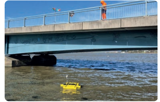
Mapping the riverbed topography and obtaining watercourse inverts
