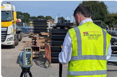
Trimble X9 on site
