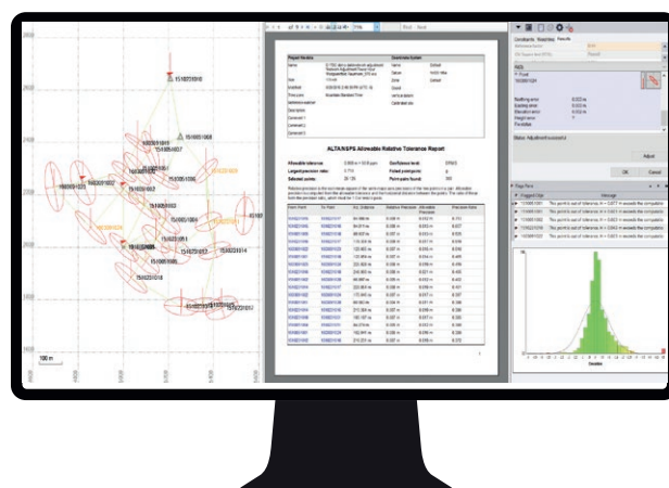
Apply a least-squares adjustment in a network adjustment
