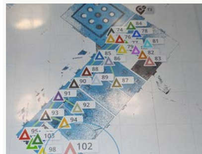
Scan data shown on the Trimble T10x Tablet
