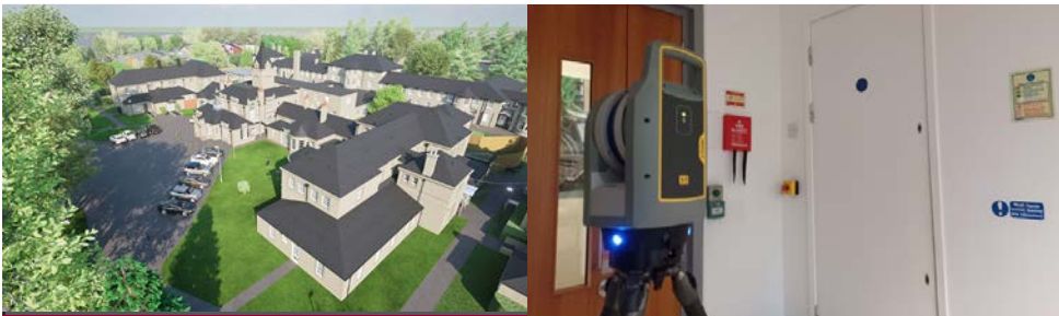
Visualisation of Warneford hospital – birds eye view (left) and the Trimble X9 in use at the hospital (right)
