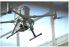
Caption: Nexys is a modular system and can be used as a handheld device as well as an attachment to a drone, ground robot, vehicle, or backpack
