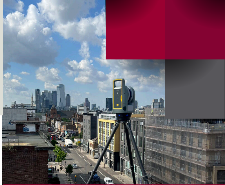
ScanPlan's Trimble X9 on a recent measured building survey project
