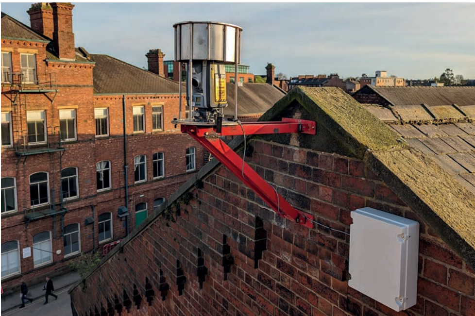
Trimble S7 Total Station and the Settop M1 housed alongside
