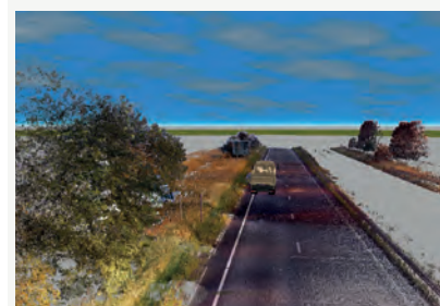
Point cloud captured by the Trimble X7
