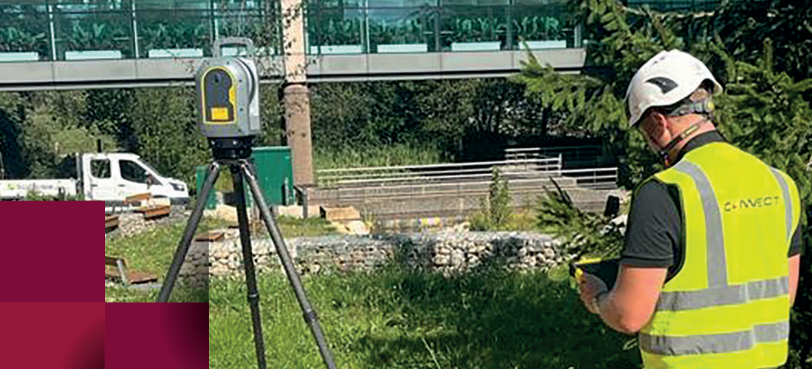
Connect Scaffolding Ltd on site with their Trimble X9 3D Laser Scanner
