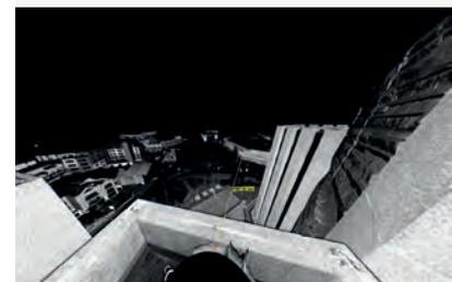
Using the X12's range to link scan data from the roof to a nearby building
