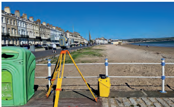
Scans were undertaken at control points using the SX10
