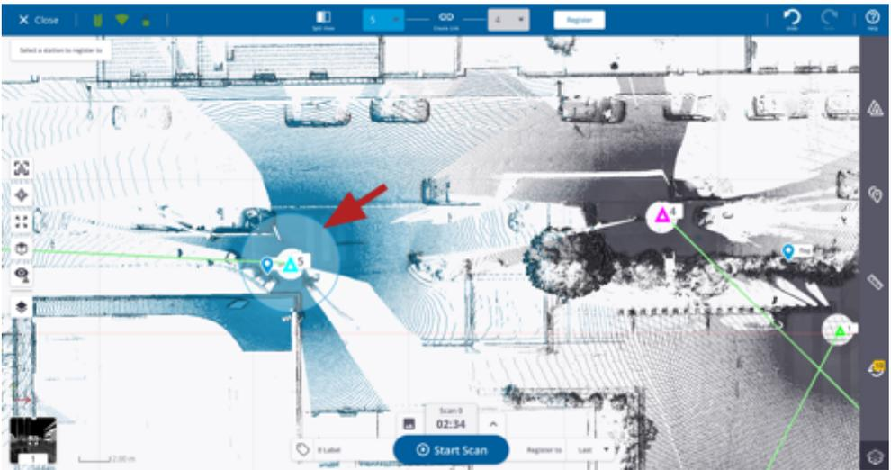
A ring manipulator appears over the moving station and the station positions of both are displayed bigger than the others. Here 5 and 4 are bigger than the rest.
