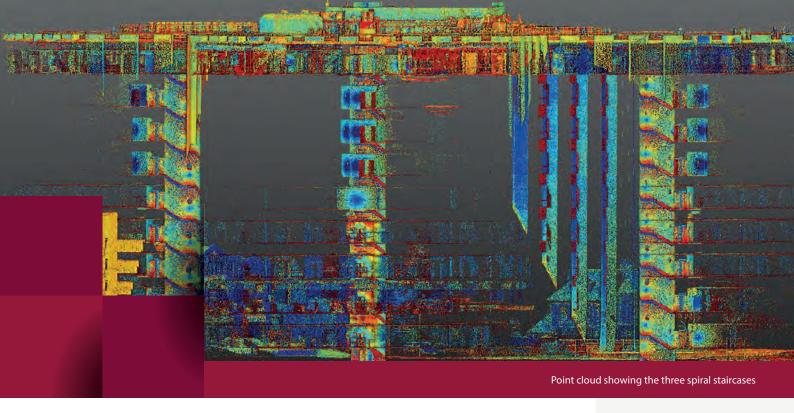
The Trimble X12 can scan at a short range of just 0.3m and also has a minimal 'blind spot' which is considerably smaller than that of other scanners, to the extent that you can see the tripod legs. This would mean that Andrew could complete the staircase scans far faster because fewer setups would be required- around half as many compared to using an alternative scanner.
