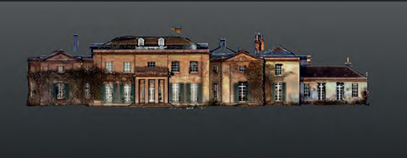
Point cloud of the private house that had a complex layout – over 200 scans were undertaken and all refined on the Trimble tablet.
