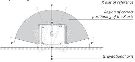
Figure 2 - Tiltmeter side view
