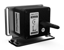
The inclinometer measures the inclination and temperature of the point where it is installed relative to the gravitational axis. By installing a system composed of these sensors it is possible to reconstruct the deformation of the structure. All inclinometers can be perfectly synchronized with each other, perfect for static load tests.
