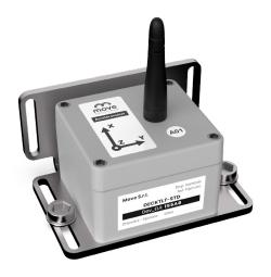
The accelerometer measures the acceleration and temperature of the exact point where it is installed in relation to the structure. It is possible to measure the vibration frequencies and carry out a modal study of the structure. All accelerometers can be perfectly synchronised with each other. Battery power supply and LoRaWAN wireless transmission.
