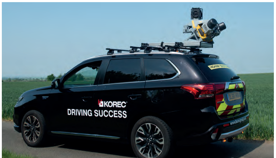
▲ KOREC Professional Service's Trimble MX9 Mobile Mapping vehicle
