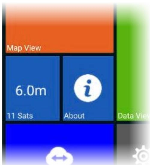
If a position fix is available and within the target accuracy in **Settings** it is **blue** and displays the precision (repeatability) of the position along with the number of satellites (Sats) used to compute the position.
