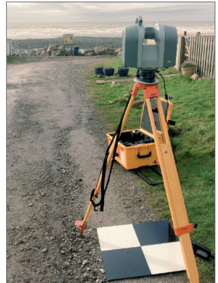
▲ The Trimble TX8 was used for Bridge 178 in St Bees
