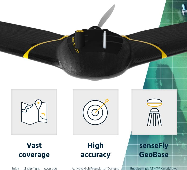
Enjoy single-flight coverage of up to 500 ha (1,235 acres) by activating eBee X's unique Endurance Extension. Activate High Precision on Demand (HPoD) RTK/PPK for absolute accuracy of down to 3 cm (1.2 in). Enable simple RTK/PPK workflows with senseFly's optional GeoBase plug-and-play GNSS receiver.
