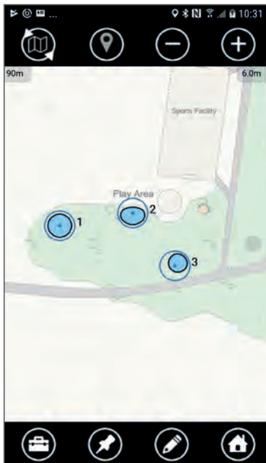
▲ Showing three captured trees – the outer rings are their root radius and crown spread.
