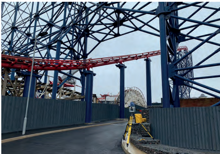
▲ The SX10 scan directly referenced control for greater accuracy
