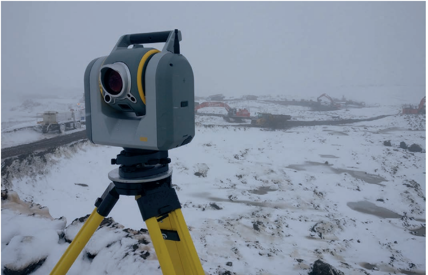
▲ Set up was in elevated positions thanks to the SX10's 600m scanning range
