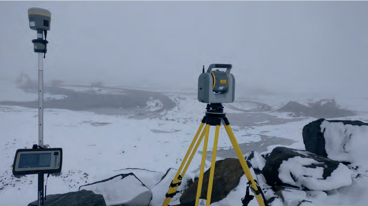
▲ Set up was in elevated positions thanks to the SX10's 600m scanning range
