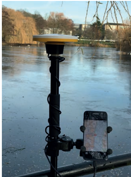
▲ Catalyst is a subscription based software GNSS receiver
