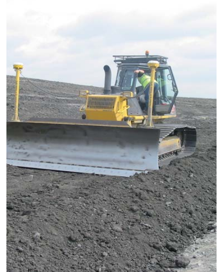
▲ The dual GPS antenna configuration computes the exact position and orientation of the machine blade for faster excavation without stakes
