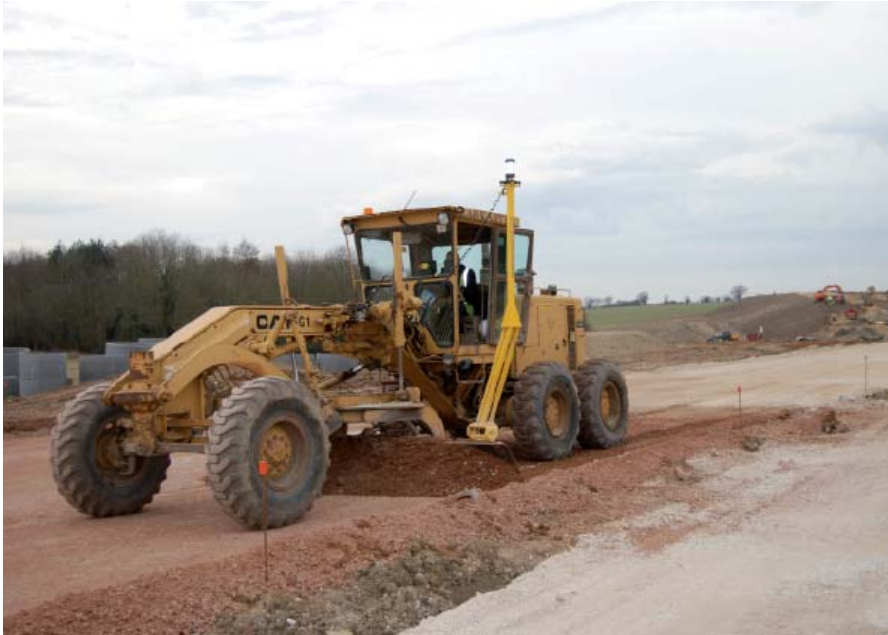
▲ Trimble's GCS900 system for graders typically delivered +/-5mm
