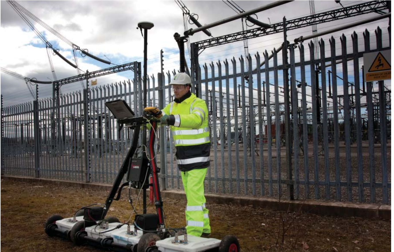
▲ The Trimble GeoXH is perfect for mapping the information recorded by Rook Services' GPR (Ground Penetrating Radar)
