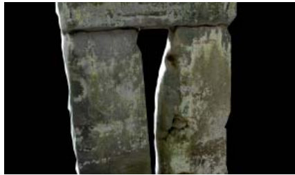
▲ Resulting scan from combining the VX Spatial Station and R8 GNSS
