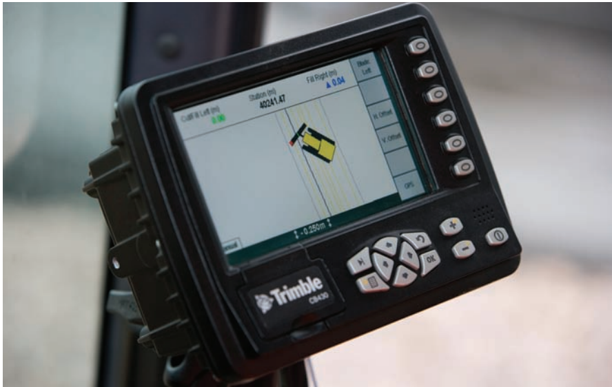
▲ Complex design data - two yellow lines show the vertical difference on the in cab screen
