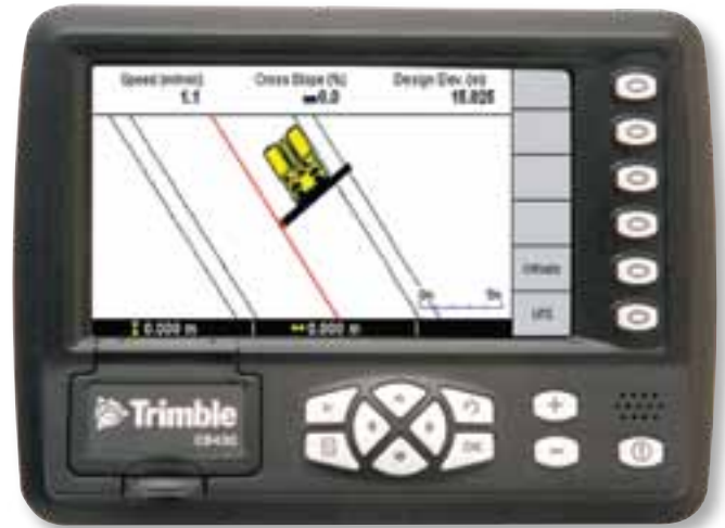
The Trimble CB430 Control Box provides a graphical display of screed position and design.
